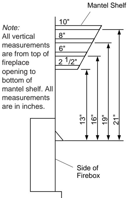
Figure 12 - Minimum Mantel Clearances for Built-In Installation
