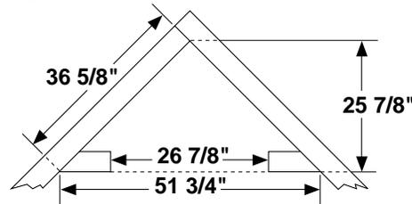
**Figure 10 - Rough Opening for Installing in Corner**
