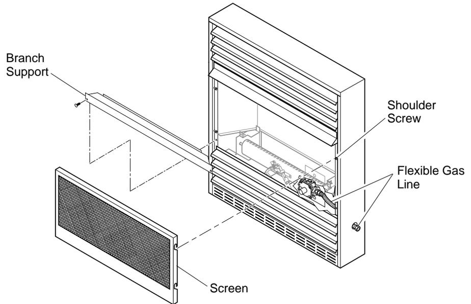
**Figure 24 - Removing Log Base Assembly From Fireplace**
