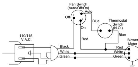
**Figure 20 - Wiring Diagram For Blower Accessory Built-In Installation**
