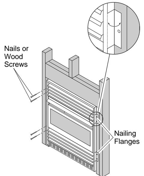
**Figure 11 - Attaching Fireplace to Wall Studs**
