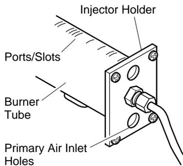
**Figure 35 - Injector Holder On Outlet Burner Tube**
