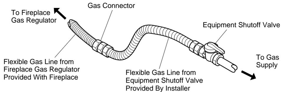
**Figure 25 - Attaching Flexible Gas Lines Together**
