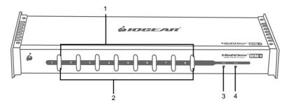
Port Selection Switches – Press a switch to access the computer attached to its corresponding port.
