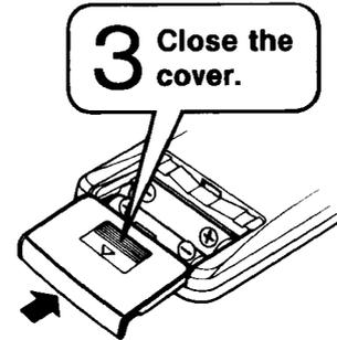
Be sure that you insert the batteries so that their positive (+) and negative (-) polarities match the polarities indicated in the compartment. Batteries installed with incorrect polarities may leak and damage.
