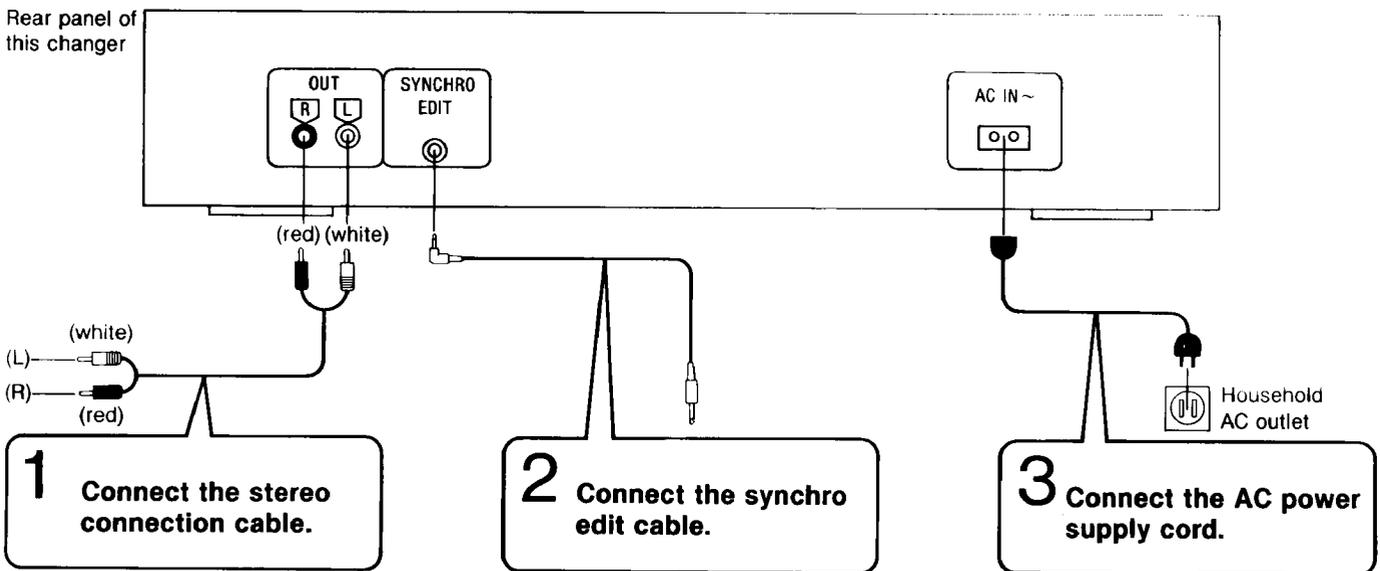
**1** Connect the stereo connection cable (included) to CD or AUX terminals of the amplifier or the receiver.
