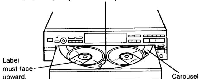
After loading discs on the two disc trays at the front position, press DISC SKIP to move the carousel. A different two disc trays will be at the front position each time DISC SKIP is pressed.
