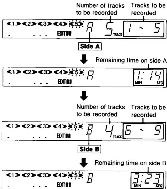
In this example, disc 5 can be recorded with tracks 1–5 on side A and tracks 6–9 on side B of the cassette tape.
