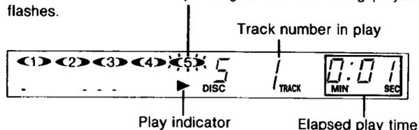
The changer plays all the tracks on all the discs in order and stops automatically when the last track on the last disc finishes playing. The first disc will be at the playing position.
