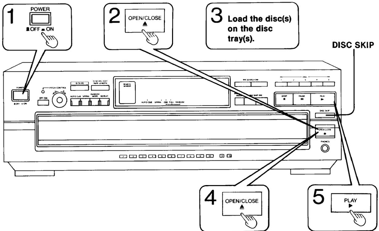
**1 Press POWER to switch on the power.**
