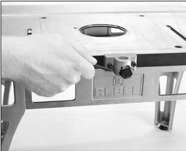
**Figure 6.** Mounting safety guard bracket.
