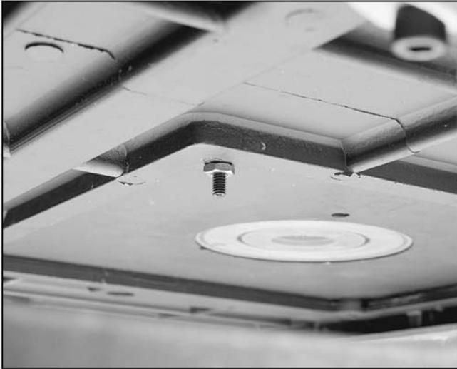
**Figure 14.** Leveling setscrew and jam nut.
