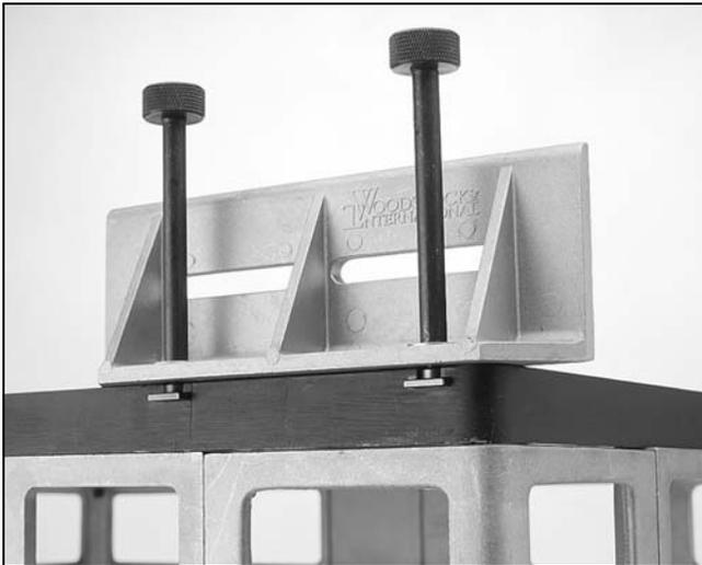
**Figure 4.** Attaching the fence.
