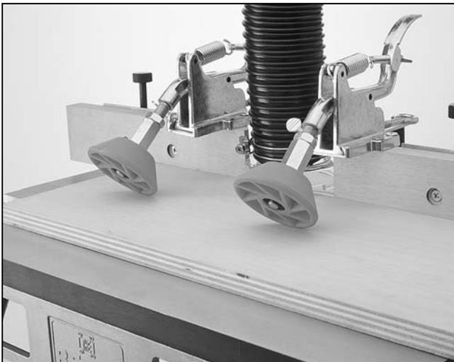
**Figure 21.** Pressure rollers.
