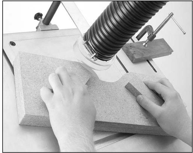
**Figure 27.** Work is supported by the guide bearing.
