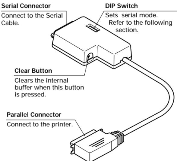
In addition to the converter, you will also need a proper serial cable. Consult with the dealer where you bought your printer if you are unsure about the type of serial cable you need for your system.
