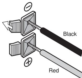
Press the button of the speaker jack and keep it pressed down as you insert the wire of the speaker cord and then release the button.
