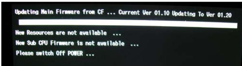
7. Power off the unit and remove the CompactFlash or SD memory card.
