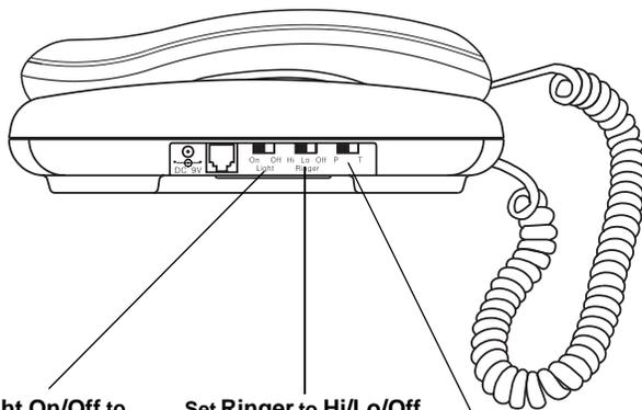
Set Light On/Off to On to turn on the neon light, or Off to turn off the light. **Note:** If you set the switch to On, the phone lights when the handset is on the base and in between rings. If you set the switch to Off, the phone only lights during each ring.
