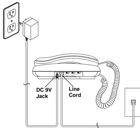
Plug one end of the supplied line cord into the jack on the back of base, and plug the cord's other end into a modular phone line jack. Insert the supplied AC adapter's barrel plug into the **DC 9V** jack on the back of the phone. Then plug the other end of the adapter into a standard AC outlet.
