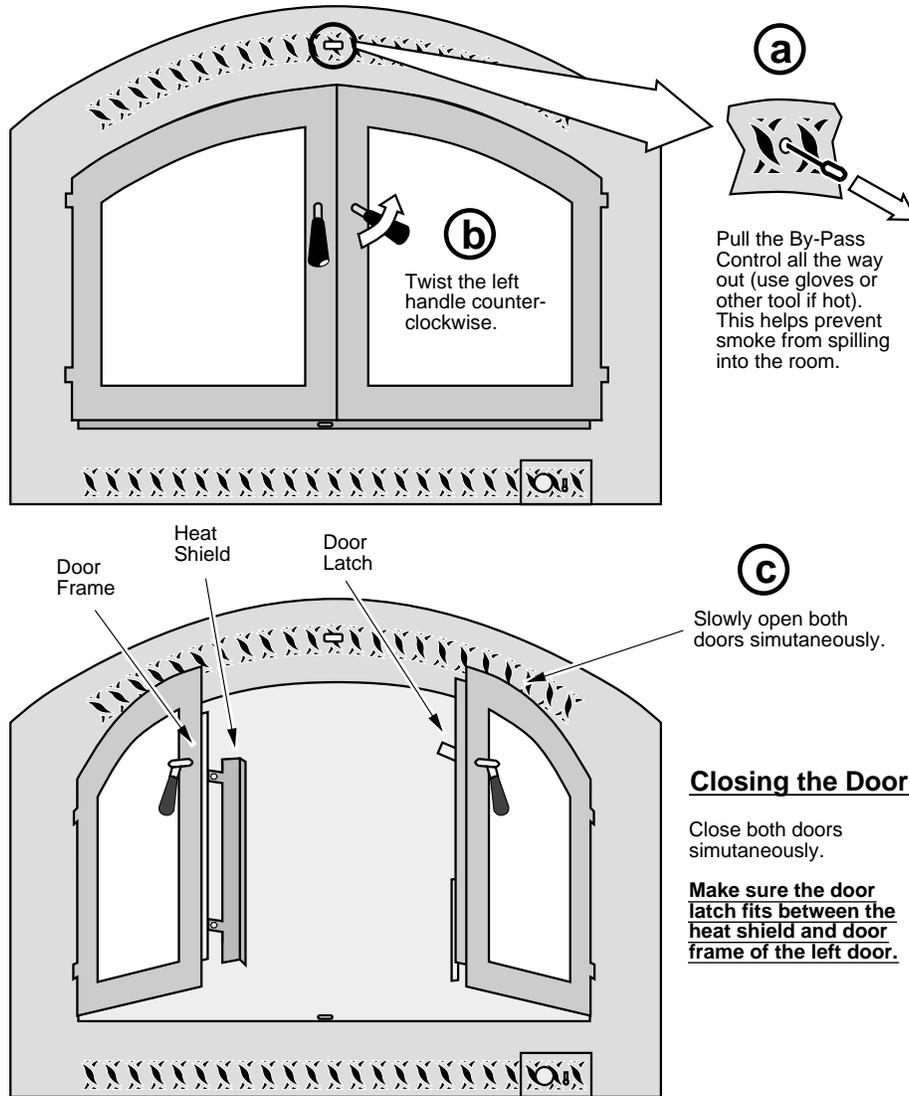
**Warning:** When closing the doors, make sure the door latch does not strike the front of the left side door. This will damage the finish on the doors.
