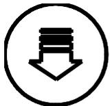
This switch changes the record displayed on the LCD to the next record on the page. When the bottom of the page has been reached the display will no longer scroll.
