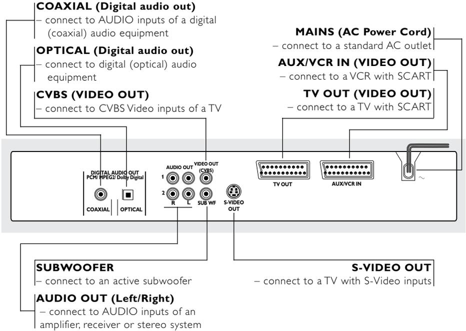
**Caution:** Do not touch the inner pins of the jacks on the rear panel. Electrostatic discharge may cause permanent damage to the unit.
