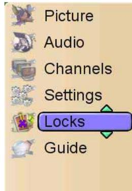
A personal identification number (PIN) will need to be created the first time the Locks menu is accessed. Enter the new PIN using the remote control, then confirm the new PIN to save it. Once the PIN has been created, the PIN Entry box will appear whenever attempting to modify the Locks menu.
