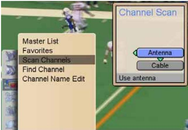
After selecting the input source, activate the Scan button to initiate scanning or cancel the scan function by selecting Don't Scan.
