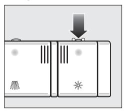
■ Press the button in the direction of the arrow until the flap springs open.
