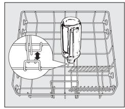
The bottle holder, e.g. for vases and baby bottles, can be inserted into the lower basket.
