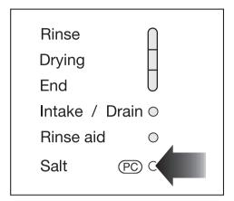
■ When the "Salt" indicator comes on, refill the salt after the program is finished.
