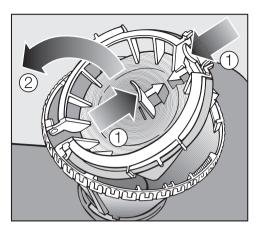
To clean the inside of the filter, the flap must be opened.
