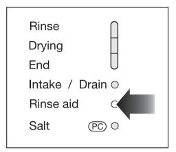
■ The rinse aid indicator on the control panel will light when the rinse aid reservoir needs refilling.
