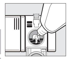
Pour liquid rinse aid into the reservoir until it its visible on the surface of the screen.
