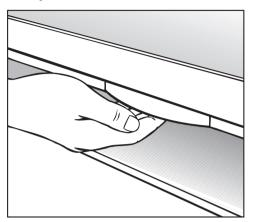
■ Press the release catch inside the door grip.
