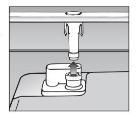
■ Pull the **lower** spray arm firmly upwards to remove.
