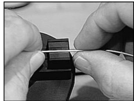
4.02 Grasp the coated fiber about .25 inches (6 mm) from the bare glass and move the fiber end onto the fiber alignment guide on the assembly tool such that the end is resting on the alignment guide outside of the splice.
