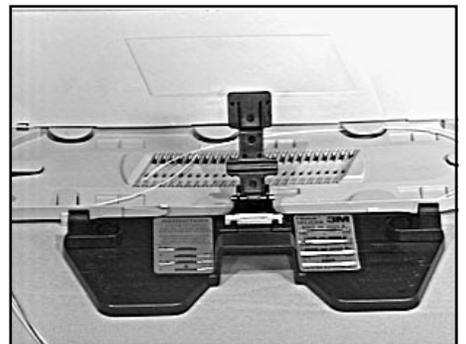
6.05 Remove the minimum amount of fiber required for fiber preparation and splicing. Remove less than one loop if possible.
