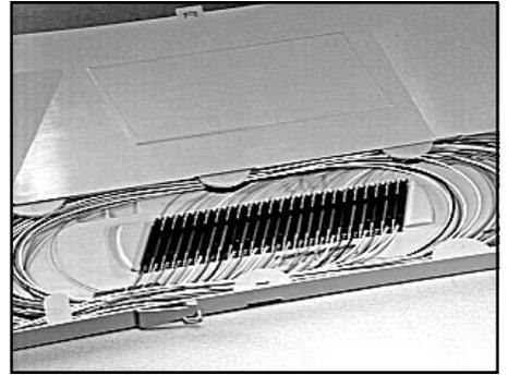
7.02 The 2524 Splice Tray fits and mounts into the 3M 2177 Fiber Optic Splice Closure, the 3M 2178 Fiber Optic Splice Case and the 3M 2190 PST Fiber Optic Splice Closure. It is also compatible with a variety of non-3M closures.
