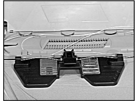
6.07 Carefully lay the splice on top of the holder without securing the splice into the holder.
