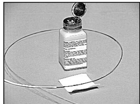
2.04 Remove Fibrlok splice from protective package. Load the splice into the assembly tool by pressing firmly at the **ends** of the splice.
