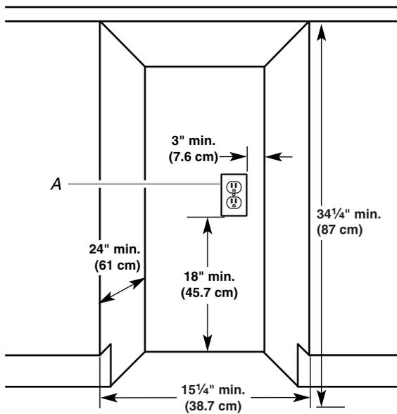
A. Grounded electrical outlet must be a minimum of 3" (7.6 cm) away from surrounding cabinets or nearby walls as shown. It can be placed either to the left or the right side of the compactor.
