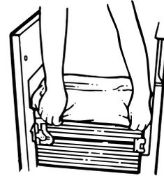
2. Lock bag in place by pulling the four prepunched holes over the bag retainer buttons. Holes will expand over the buttons without damaging the bag.
