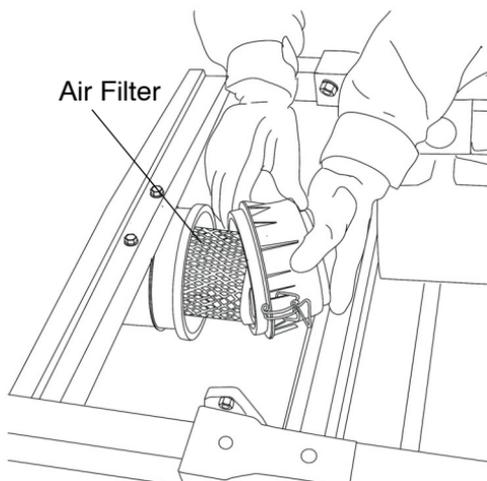
5. Inspect the air box for oil or water deposits. If present, drain them into a suitable container.
