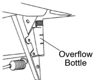
**NOTE:** If coolant must be added often, or if the overflow bottle runs completely dry, there may be a leak in the system. Have the cooling system inspected by your Polaris dealer.
