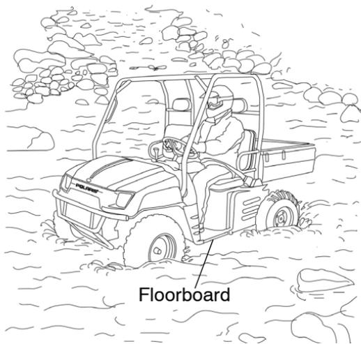
**NOTE:** After running your vehicle in water, it's critical that you perform the services outlined in the Periodic Maintenance Chart beginning on page 52. Give special attention to engine oil, transmission oil, front and rear gearcases, and all grease fittings.
