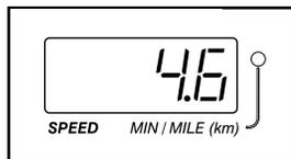
Each time a button is pressed, the speed setting will change by 0.1 mph; if a button is held down, the speed setting will change in increments of 0.5 mph. To change the speed setting quickly, press the Quick Speed buttons. **Note: The console can display speed and distance in either miles or kilometers. For simplicity, all instructions in this section refer to miles.**
