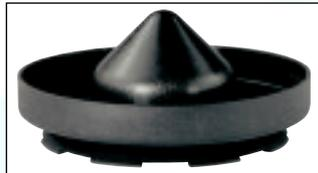
The combination of conical flow diffuser and a drainage layer wrapped under the lower endcap allows airflow through the lowest section of the element, which is not possible on conventional filters due to the position of the “wet band”.
