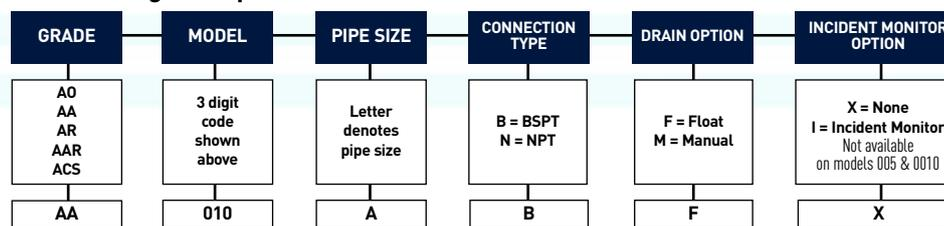
**Note:** AO / AA grade filters for use up to 16 bar g (232 psi g) are supplied with a float drain [F] as standard. For pressures of 16 to 20 bar g (232 to 290 psi g) a manual drain [M] must be used. ACS / AR / AAR grade filters are supplied with a manual drain [M] as standard.
