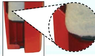
Drainage ribs cast into the filter bowl compress the lower part of the filter element, allowing bulk liquid to rapidly drain from the filter element through capillary action.
