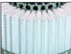
Deep bed pleating of the filter media reduces the air flow velocity within the media, which in addition to improving the filtration performance of the element, significantly reduces pressure losses and energy consumption.
