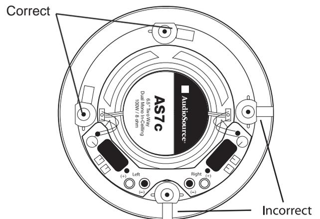
With the grill removed, place the speaker in the ceiling opening. Make sure that the speaker wire is not hanging against the speaker where it can vibrate and rattle as the speaker reproduces your music.
