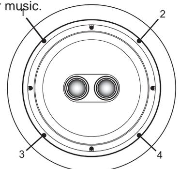
Tighten all four of the mounting screws in the same manner until the speaker is properly aligned and held tight to the wall surface. *Caution: Do not over tighten!*
