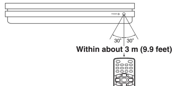
Distance: About 3 m (9.9 feet) from the front of the remote sensor
