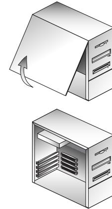
Select an available PCI slot and, if necessary, remove its cover plate.
