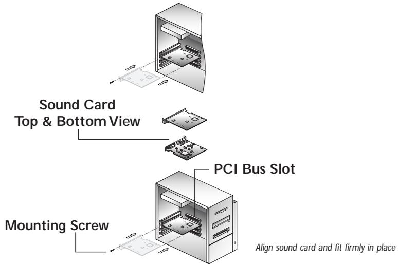
Use the screw from the slot cover to secure the sound card to the frame of the computer chassis, but do not over-tighten. Securing the card assures proper grounding.
