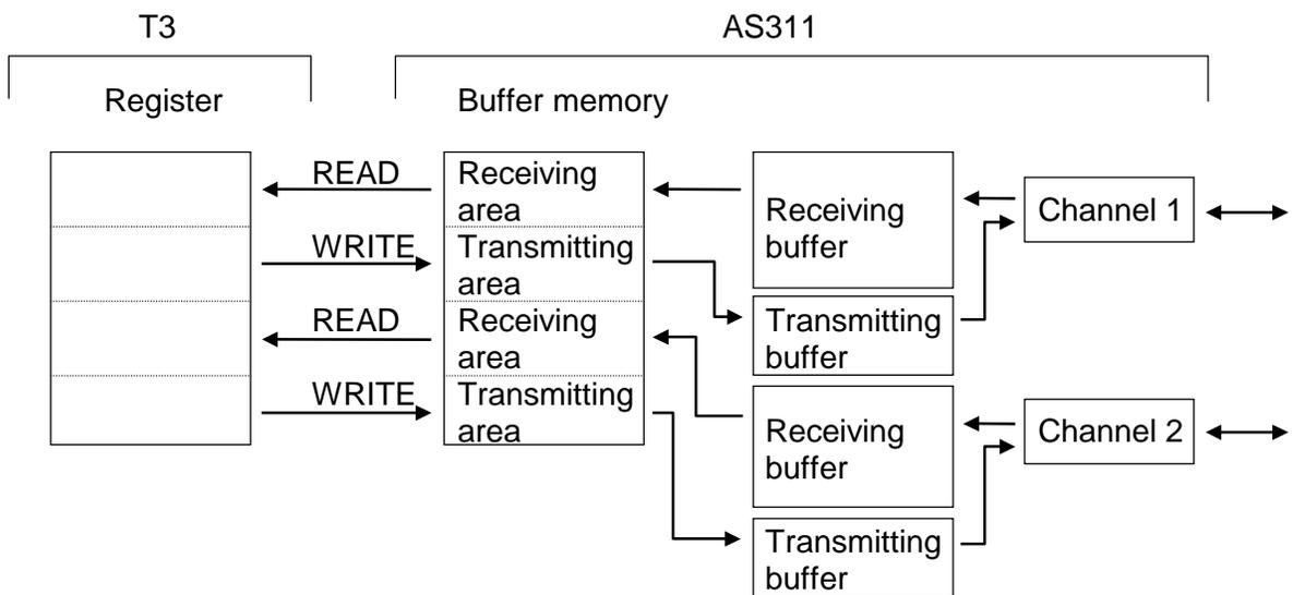
Here, a message (one set of transmission characters) means a string of ASCII characters which is ended by specified trailing code. The default setting of the trailing code is CR (carriage return code = H0D).
