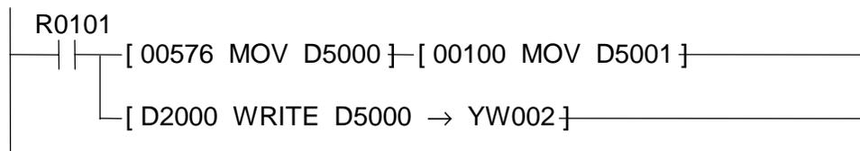
When R0101 is ON, 100 words of data starting with D2000 (D2000 to D2099) are written into the buffer memory address 576 and after of the AS311 which is allocated to YW002.
