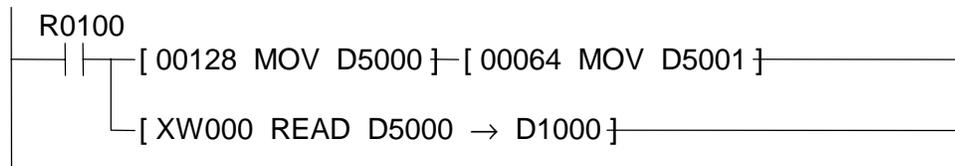
When R0100 is ON, 64 words of buffer memory data starting with address 128 are read from the AS311 which is allocated to XW000. And the data are stored in D1000 and after.
