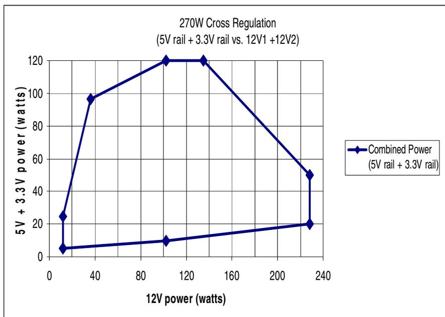
**Figure 5 Cross Loading Graph for 270W Configuration**
