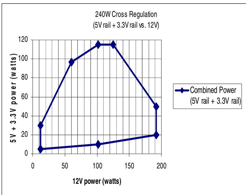
**Figure 4. Cross Loading Graph for 240W Configuration**
