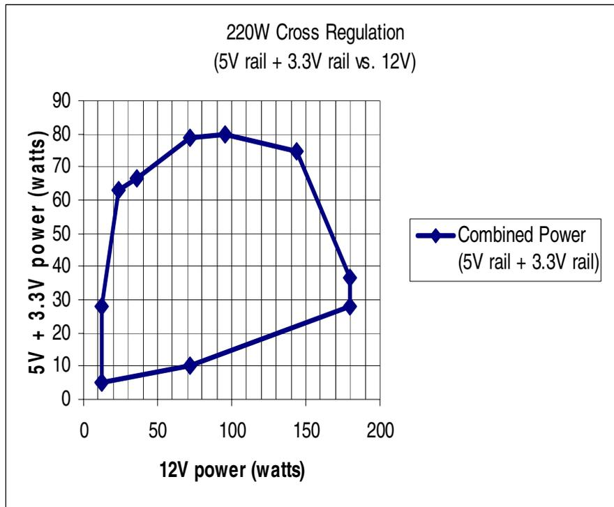
**Figure 3. Cross Loading Graph for 220W Configuration**
