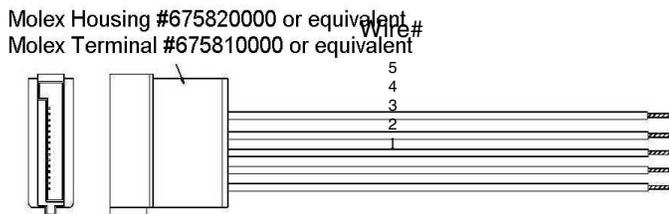
**Figure 15. Serial ATA Connector**
