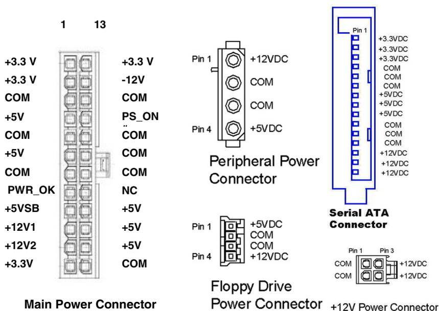
Figure 14. TFX12V Connectors (Pin-side view, not to scale)
