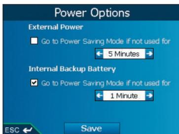
*Note: if you are not going to be using the iCN for an extended period of time, switch the **Battery Switch** to **OFF** to save battery power.*
