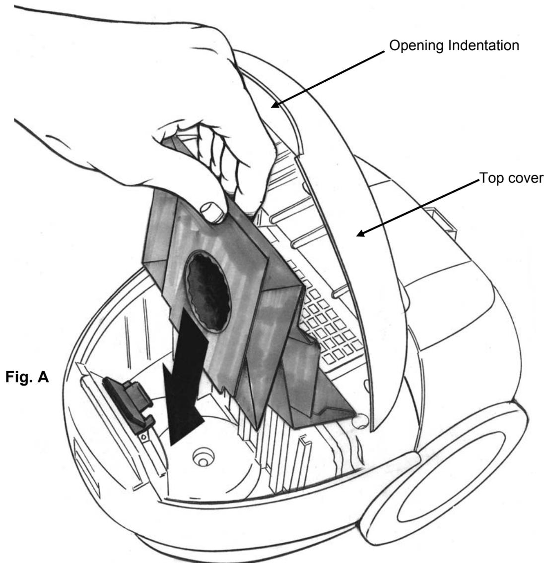
2. Hold the bag in your hand and insert it into the slot on the bottom, (Fig. A)
