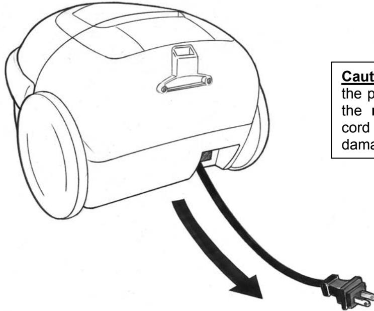
**Caution:** Do not pull the power cord beyond the **red mark** on the cord as doing this will damage the cord.
