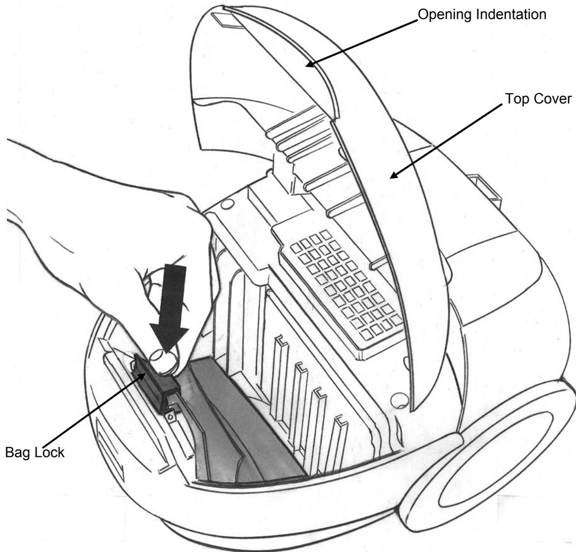
4. Lock the bag in its place with the lock as shown in Fig. C.
