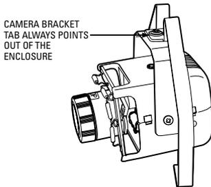
**Ceiling Mounting:** The camera bracket tab points out of the enclosure, and the top of the camera is pointed in the opposite direction.
