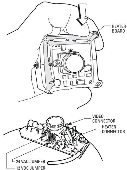
3. If the heater is installed, plug the heater connector from the camera into the mating connector inside the base. Plug the video connector from the camera into the mating connector inside the base.
