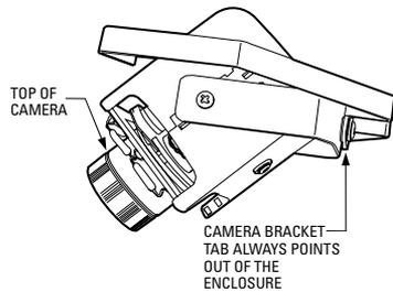
**Wall Mounting:** The camera bracket tab points out of the enclosure, and the top of the camera points up towards the tab.
