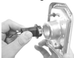
2. Remove the tail light housing hardware so the housing can be removed from the car.
