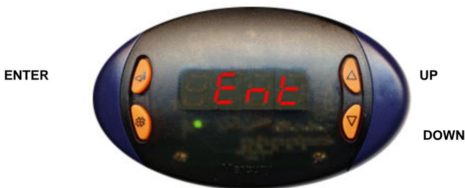
To enter set-up mode, hold the Enter and Down buttons together for approximately 3 seconds until the message “Ent” appears on the display. Now press the Enter button again to enter the function menu. IO will be displayed. Scroll up or down to go through the list.
