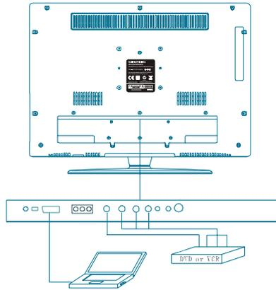
1. Connect the TV RF source to the RF IN port. TVRF signal including: Receiving antenna /satellite TV/CATV net. You can use 75Ω coaxial cable to connect the outdoor antenna.
