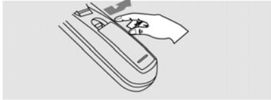
2. Install the battery into the battery tray.
