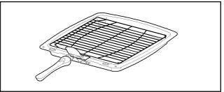
To remove the handle, slide the handle to the right and lift the handle away from the cut out on the grill pan.
