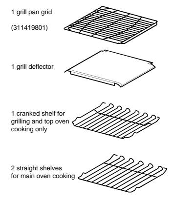
The grill deflector sits above the grill element and prevents fat splashing onto the grill roof. The deflector may be easily removed for cleaning.
