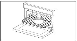
When cooking cakes, pastry, scones, bread, etc., place the tins or baking trays centrally on the shelf directly below the element.  DO NOT place dishes directly onto the oven base as it becomes very hot and damage may occur.
