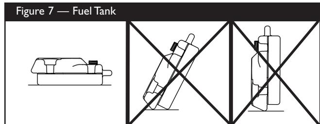
To place the fuel tank back on the unit, follow these same steps in reverse order. Make sure the four large plastic wing nuts are tightened securely.
