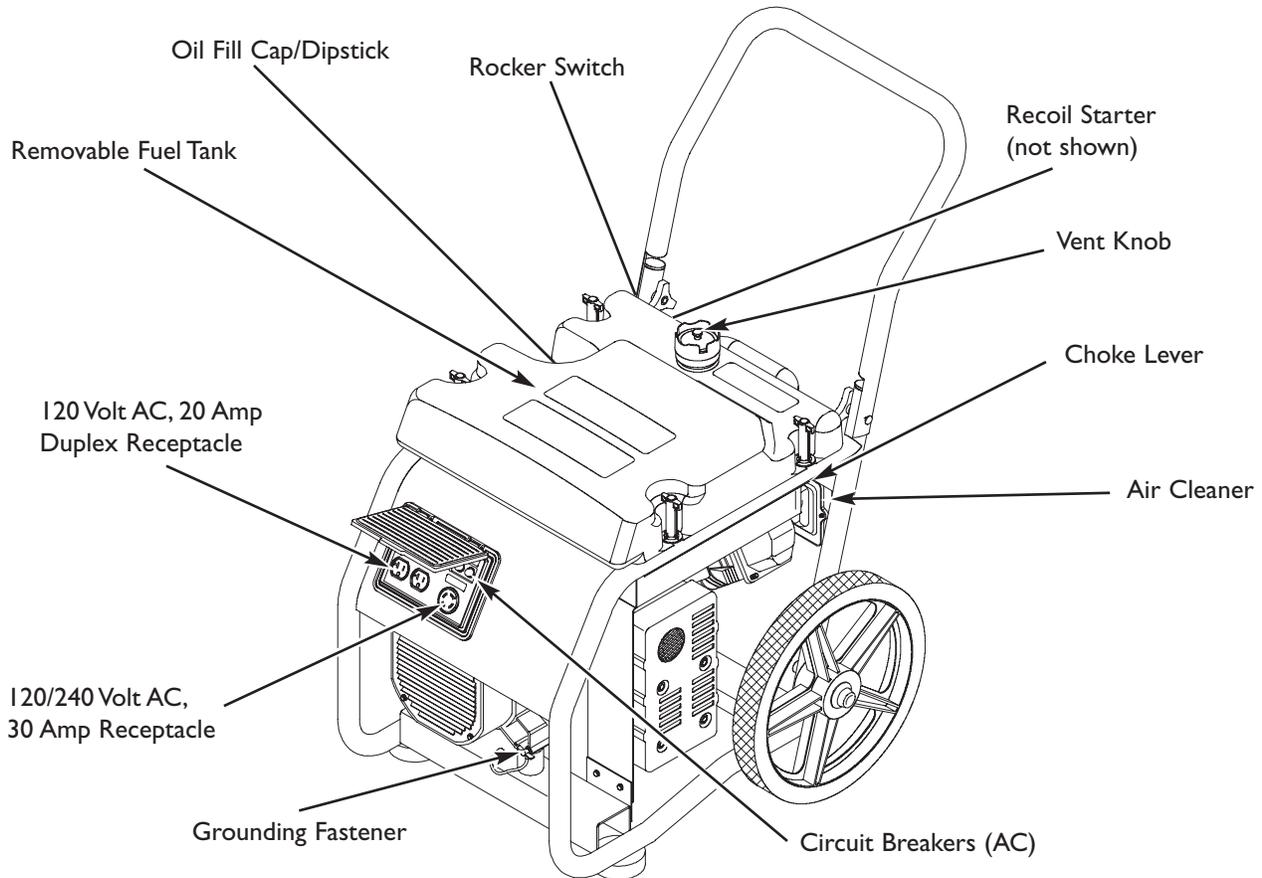
**120 Volt AC, 20 Amp, Duplex Receptacle** — May be used to supply electrical power for the operation of 120 Volt AC, 20 Amp, single phase, 60 Hz electrical lighting, appliance, tool and motor loads.
