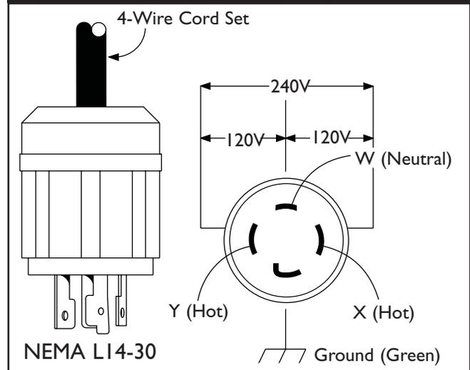
This receptacle powers 120/240 Volt AC, 60 Hz, single phase loads requiring up to 2,775 watts of power at 23.1 Amps for 120 Volts; 5,550 watts of power (5.55 kW) at 23.1 Amps for 240 Volts. The outlet is protected by a push-to-reset circuit breaker.
