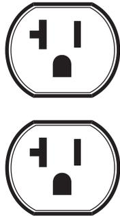
Use each receptacle to operate 120 Volt AC, single-phase, 60 Hz electrical loads requiring up to 2,400 watts (2.4 kW) at 20 Amps of current. Use cord sets that are rated for 125 Volt AC loads at 20 Amps (or greater).
