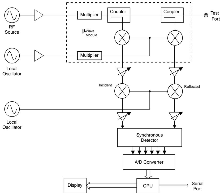
**Figure 2.** Site Master Block Diagram
