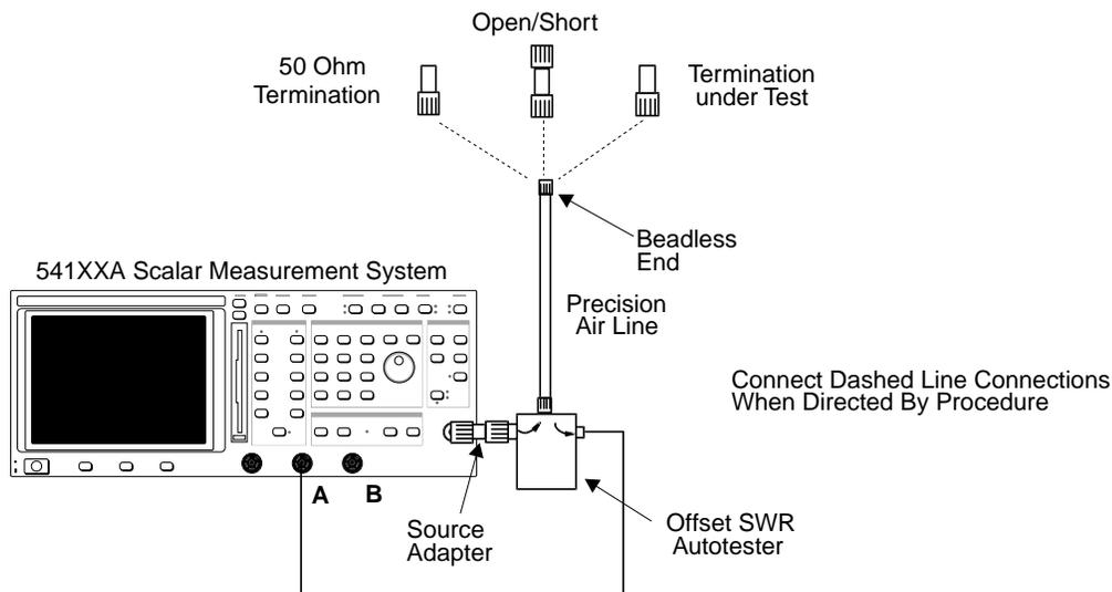
**Figure 4.** 541XXA Precision Return Loss Test Setup
