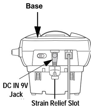
4. Place the handset on the base and charge continuously for 15-20 hours before using the phone.
