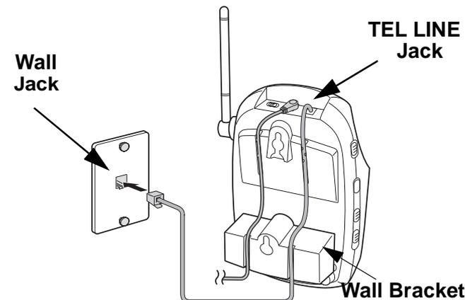
**Note:** The illustration shows the wall-mount bracket attached. See page 9 of your Owner's Manual for how to attach and use the bracket.
