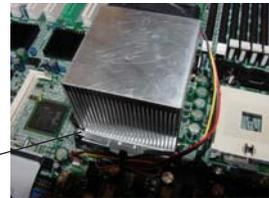
10. Connect the three wires of the CPU fan to the respective CPU fan connector.
