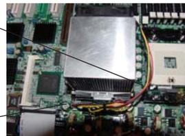
Figure 2-1. PGA604 Socket: Empty and with Processor Installed
