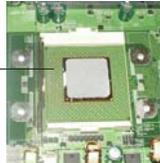
8. Apply the proper amount of thermal glue to the CPU die and place the heatsink and fan on top of the CPU.
