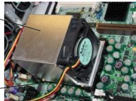
9. Secure the heatsink by locking the retention clips into their proper position.
