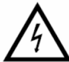
Lightning Flash Symbol, with "The Lightning Flash with arrowhead symbol within an equilateral triangle, is intended to alert the user to the presence of uninsulated "dangerous voltage" within the product enclosure that may be of sufficient magnitude to constitute a risk of shock to persons"
