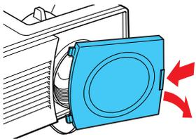
Be sure to remove the lens cover when the power is turned on. If it is left on, it could become deformed due to heat.
