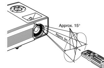
When operating the remote control from behind the projector, the laser light is reflected on the projecting surface and may travel a shorter distance to reach the projector depending on the shape and material of the projecting surface.
