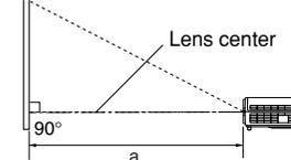
a is the distance (m) between the lens and the screen, and corresponds to a range of 1.07 m to 11.09 m.
