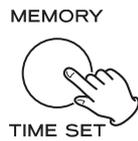
In the stop mode, press the MEMORY button repeatedly. The track number and program number will be shown on the display.
