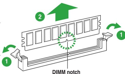
2. Remove the DIMM from the socket.
