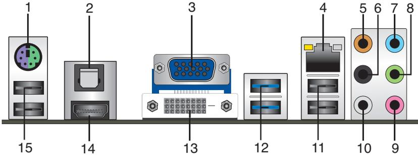
1. **PS/2 Keyboard/Mouse combo port.** This port is for a PS/2 keyboard/mouse.
