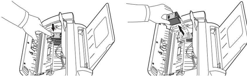
**5** To load the cartridge insert the cartridge below the metal clip and pointing down at the front. When the cartridge is pushed to the back of the cartridge carrier lift the front of the cartridge up until it clicks into place.
