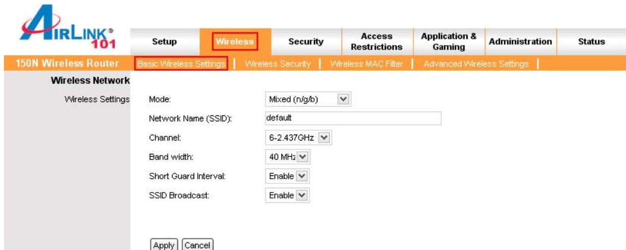
The screenshot shows the web interface of an Airlink 101 wireless router. The top navigation bar includes tabs for Setup, Wireless, Security, Access Restrictions, Application & Gaming, Administration, and Status. The 'Wireless' tab is selected. Below this, there are sub-tabs for Basic Wireless Settings, Wireless Security, Wireless MAC Filter, and Advanced Wireless Settings. The 'Basic Wireless Settings' sub-tab is active, displaying the following configuration:
