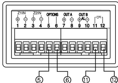
**Note:** Industry standard designation for RS-485 lines is A and B. Some equipment manufacturers use a non-standard designation of plus and minus. The association of A to minus and B to plus is based on a sample of devices marked as plus and minus and is not intended to represent ALL such labelled devices. Final responsibility for correct identification of leads and terminals rests with the user/installer and the manufacturer of the other device(s) installed in the system.
