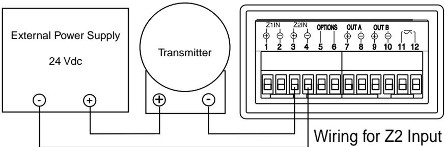
For three or four wire transmitters follow the wiring instructions provided with your transmitter.
