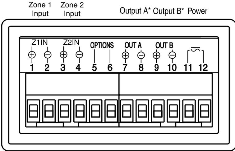
\* Output A is assigned to Zone 1 Input and Output B is assigned to Zone 2 Input. If necessary, the input/output relationships may be reversed. See *SP id* in Secure Menu.
