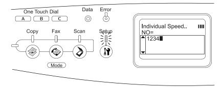
To correct a number while entering it, use the ◀ button to go back one character or the \$\preces Reset button to delete.
