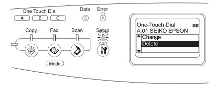
7. Press the ▼ button to select **Yes** for confirmation, then press the ▶ button. The recipient assigned for the one-touch dial is deleted.
