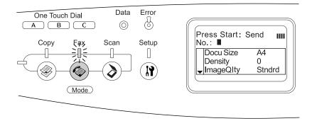
If you press the **S** Fax button while in Fax mode, the screen returns to the Print mode. You can still scan and print from your computer in Fax mode.
