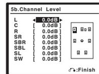
Adjust the level of each speaker as the test tone is emitted.<sup>4</sup>
