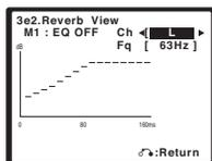
This appears according to the setting you chose in **Reverb Measurement** (step 3 above). Use the  $\leftarrow/\rightarrow$  buttons to select the channel and the frequency you want to check. Use the  $\uparrow/\downarrow$  buttons to go back and forth between the two. Note that the markers on the vertical axis indicate decibels in 2dB steps.
