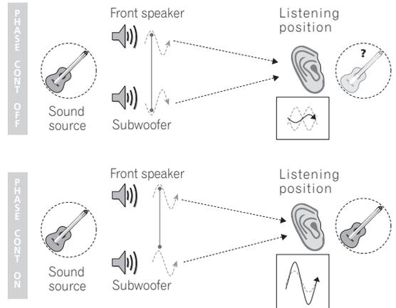
Phase Control technology provides coherent sound reproduction through the use of phase matching<sup>4</sup> for an optimal sound image at your listening position. The default setting is on and we recommend leaving Phase Control switched on for all sound sources.
