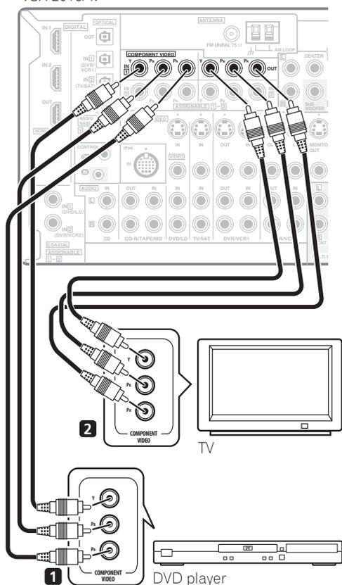
**1 Connect the component video outputs of your source to a set of ASSIGNABLE COMPONENT VIDEO inputs.**
