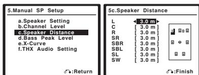
**2 Adjust the distance of each speaker using the ←/→ buttons.**
