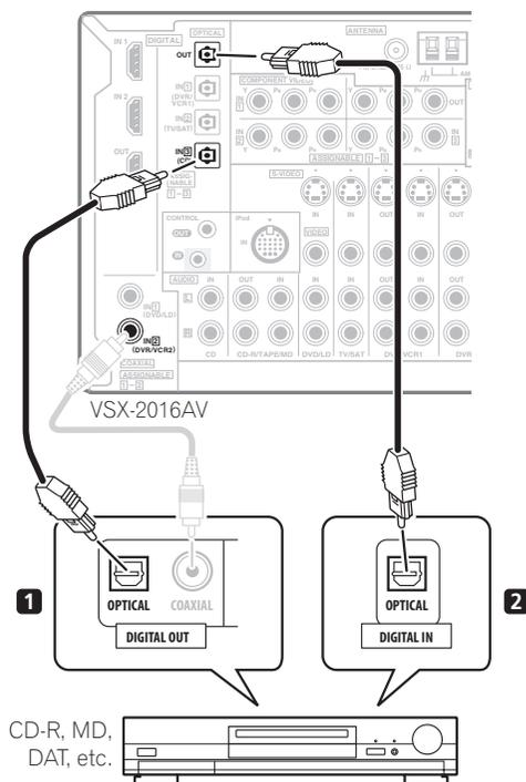
**1 Connect an optical-type<sup>1</sup> digital audio output on your digital component to the DIGITAL 3 (CD) input.** Use an optical cable for the connection.
