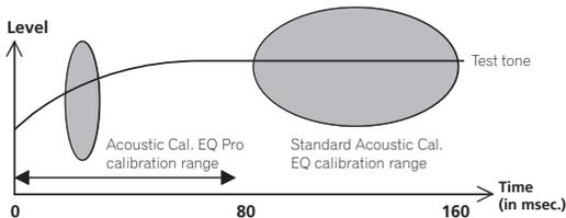
As soon as audio is output from your speaker system, it is influenced by room characteristics, such as walls, furniture, and the dimensions of the room. The sooner the frequency analysis, the less it is influenced by the room. We recommend an earlier time setting of 20 ms to 40 ms to compensate for two major factors that will influence the sound of most rooms:
