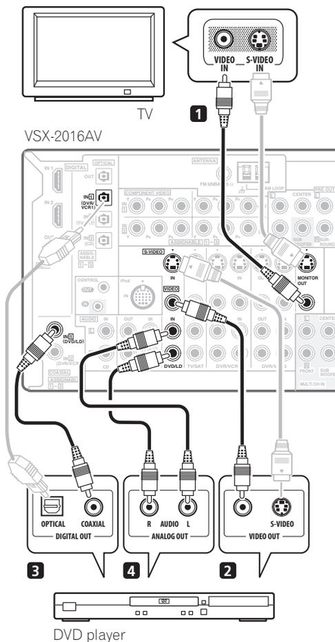
The diagram shows a basic setup of this receiver together with a TV and DVD player, with S-video or composite video connections. Different TVs and DVD players may offer alternative connections. See also *Using the component video jacks* on page 14 if your TV and/or DVD player has component video inputs/outputs. If your DVD player offers multichannel analog audio outputs, see *Connecting the multichannel analog inputs* on page 51.
