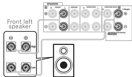
Since both front and surround back speaker terminals output the same audio, it doesn't matter which set (front or surround back) is powering which part (**High** or **Low**) of the speaker.
