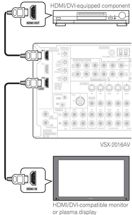
**1 Use an HDMI cable to connect the HDMI IN/2 interconnect on this receiver to an HDMI output on your HDMI component.**
