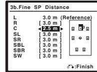
Listen to the reference speaker and use it to measure the target channel. From the listening position, face the two speakers with your arms outstretched pointing at each speaker. Try to make the two tones sound as if they are arriving simultaneously at a position slightly in front of you and between your arm span.<sup>1</sup>
