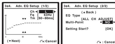
Use the  $\leftarrow/\rightarrow$  buttons to select the channel, frequency, and time setting. Use the  $\uparrow/\downarrow$  buttons to switch between them.
