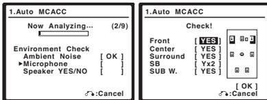
If you see an error message (**ERR**) in the right side column (or the speaker configuration displayed isn't correct), there may be a problem with the speaker connection. If selecting **RETRY** doesn't work, turn off the power and check the speaker connections. If there doesn't seem to be a problem, you can simply use **↑/↓** to select the speaker and **←/→** to change the setting (and number for surround back) and continue.
