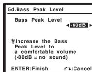
Set the bass peak level gradually, then press **ENTER** at the point just before the tone starts to distort.<sup>1</sup> The display on the receiver shows **RESUME** while the volume returns to its original position, then you automatically return to the main Bass Peak Level menu.
