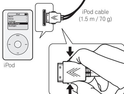
**1 Switch the receiver into standby then use the supplied iPod audio control cable<sup>2</sup> to connect your iPod to the iPod jack on the rear of the receiver.**
