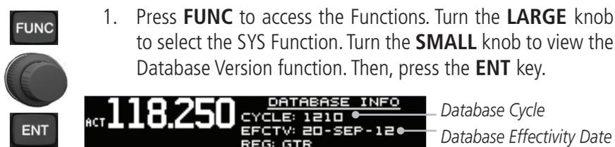
1. Press **FUNC** to access the Functions. Turn the **LARGE** knob to select the SYS Function. Turn the **SMALL** knob to view the Database Version function. Then, press the **ENT** key.
