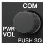
Turn the GTR 225 on by either turning the **Power/Com Volume/Squelch** knob clockwise to turn the power on or, if installed, turning on the master switch that powers the radios.
