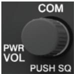
The **Power/Com Volume/Squelch** knob located in the top left corner of the bezel controls audio volume for the Com radio. Rotating the knob clockwise past the detent turns power on and counter-clockwise turns power off. When the Com radio is active, press the **Power/Com Volume/Squelch** knob to toggle automatic squelch control On/Off for the Com radio.
