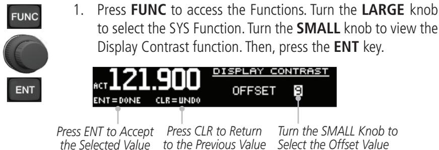
1. Press **FUNC** to access the Functions. Turn the **LARGE** knob to select the SYS Function. Turn the **SMALL** knob to view the Display Contrast function. Then, press the **ENT** key.
