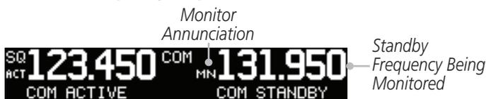
Figure 2-2 Com Frequency Monitor Annunciation
