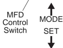
MFD settings can be made with the engine running or with the engine off. If the engine is off, make sure the stop switch is pressed down, and turn the ignition key to the START position briefly to activate the gauge. The gauge will illuminate for about 90 seconds.
