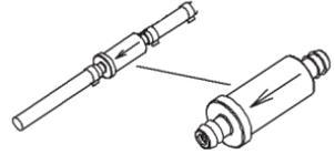
**Tip:** The direction of the arrows indicates the direction of flow through the filter.
