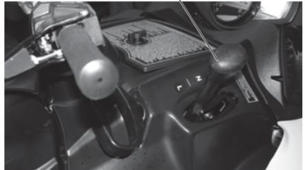
**NOTICE:** Towing a disabled snowmobile with the transmission in gear can result in serious damage to the engine and drive system. Always place the transmission of the disabled snowmobile in neutral before towing.
