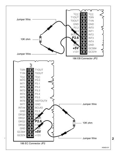
Figure 3-2. Jumper Assembly for Flash Downloading
