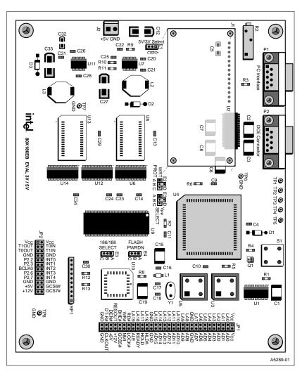
Figure 2-1. Intel 186 EB Evaluation Board Layout
