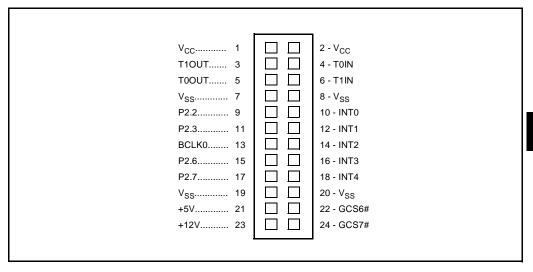
Figure 3-7. 186 EB Peripheral Expansion Connector JP2 (24 pin)
