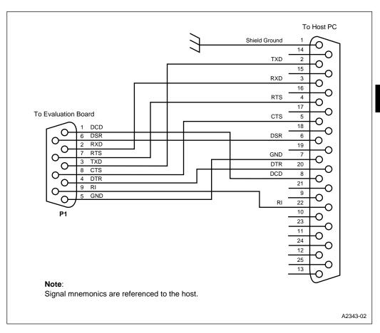
Figure 3-5. 25-Pin to 9-Pin Adaptor
