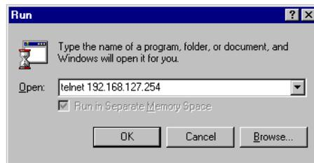
2. Type `telnet [IP_address]` in the **Open** text input box, where `[IP_address]` is the IP address of the NPort Server Pro you intend to configure. Click **OK** to continue.
