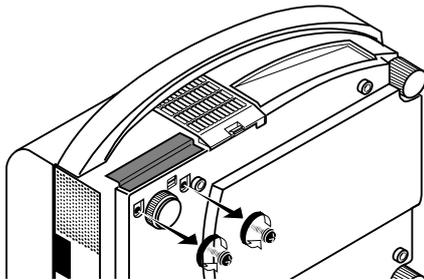
3. Remove the slot cover by pushing up on the catch of the cover with a flat-head screwdriver until you feel it detach.
