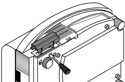
4. Insert the optional viewer board into the slot. Be sure to push the board until the board is securely fitted.
