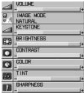
Provides access to controls for your image and sound. Use the "Select" button on the projector cabinet or (▲) (▼) buttons on your remote control to highlight the menu for the item you want to adjust. The volume, image mode, keystone, brightness, contrast, color, tint and sharpness controls are available for Video or S-Video sources.
