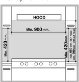
• If the cooker is installed underneath a wall cabinet, there must be a minimum distance of 420 mm between this cabinet and the top of the hob.
