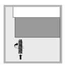
If it is necessary to level the appliance, screw the adjustable feet into the places provided on each corner of the base of the cooker (see figure).
