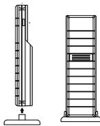
We have provided a mounting plate that you can attach to a surface with the supplied screws. The Sensor can be positioned on a flat surface by securing the stand to the bottom by gently pushing the bottom of the Sensor onto the holding pegs of the stand until they click into place in the grooves on the Sensor.
